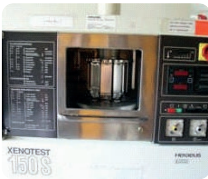
Test chamber for UV test.
