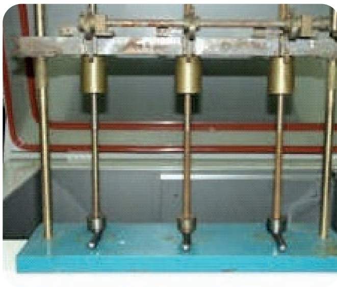
Test equipment for cold impact test.
