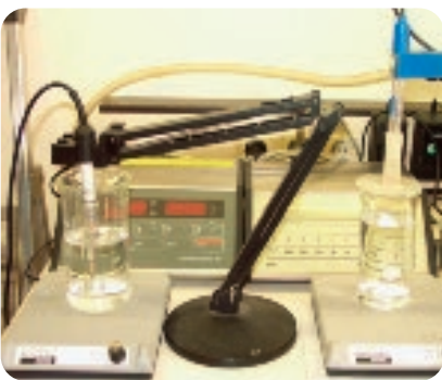
Equipment for measuring light conductivity and pH-value (halogen free).
