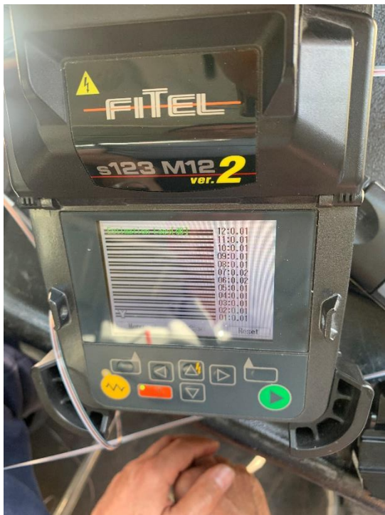
Figure 25 Screen shot of a flat ribbon splice on the Fitel splice machine
