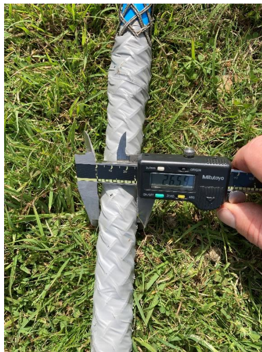
Figure 5 - FlexRibbon™ cable diameter measured with the hauling sock fitted.
