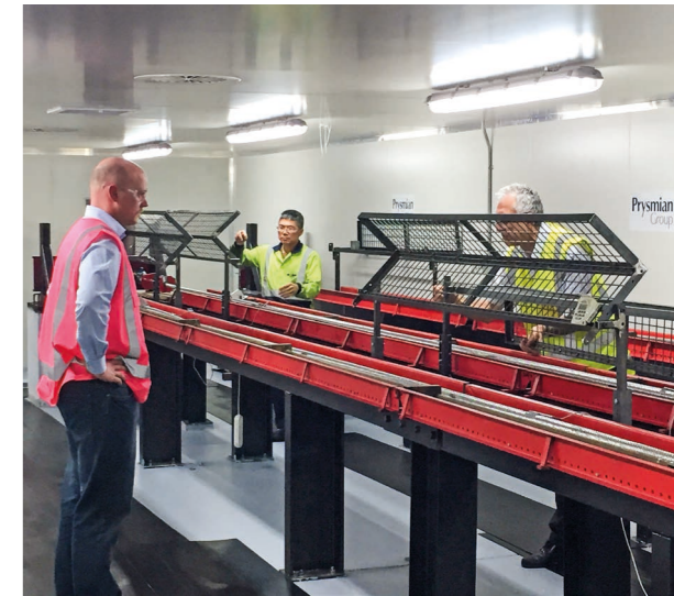
Prysmian's new 'creep test' lab aids line design by predicting long-term conductor behaviour
